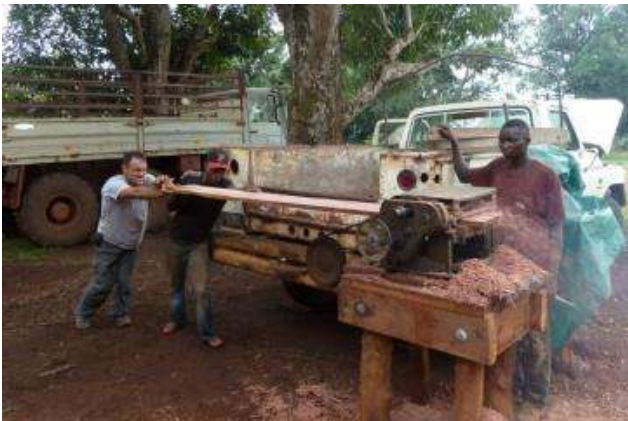
Steve and some workmen using a planer powered by Dad Pontier's pick-up which was still up here
